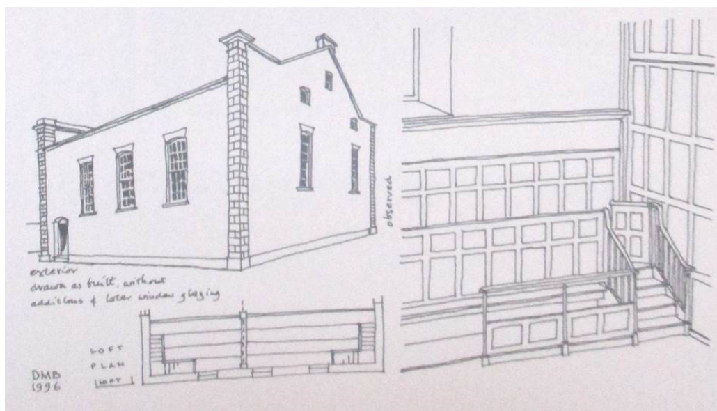
Figure 3: Elevations and internal details of the 1823 Meeting House (from Butler, Vol. 1, p. 169)
